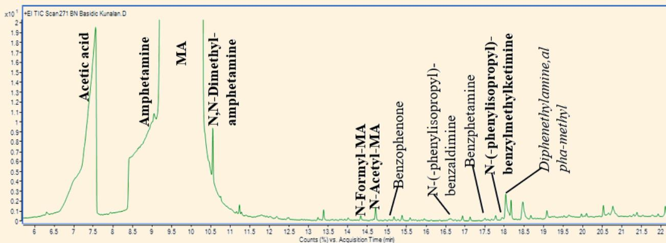
Fig. 5. Typical TIC of seized MA under basic extraction
