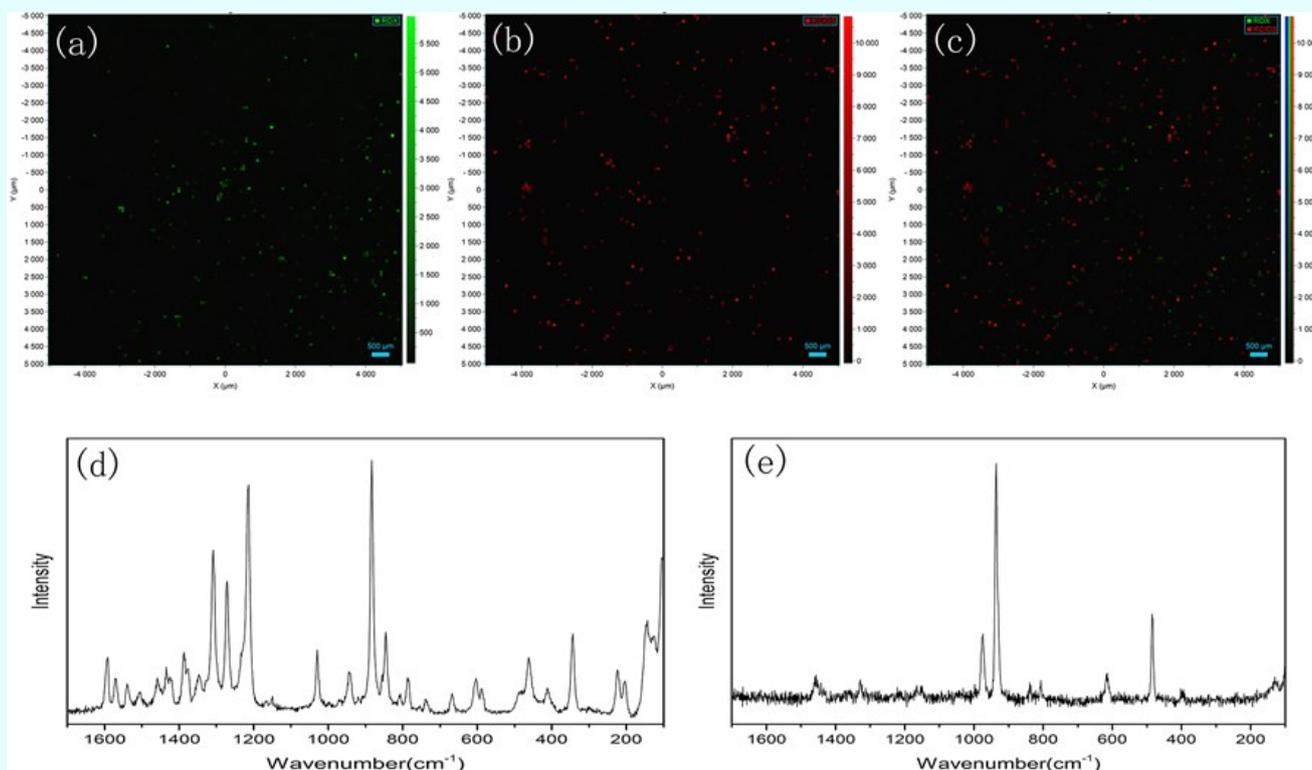
Figure 3: The distribution of explosive particles by selecting the characteristic Raman bands. (a) RDX distribution ( $870\text{--}900\text{ cm}^{-1}$ ); (b)  $\text{KClO}_3$  distribution ( $470\text{--}500\text{ cm}^{-1}$ ); (c) RDX (green) and  $\text{KClO}_3$  (red) distribution; (d) and (e) is the Raman spectra of RDX and  $\text{KClO}_3$  particles on the sticky side of the tape respectively. (Spectral acquisition time: 500 ms; acquisition times: 1; laser power: 13.5 mW).
