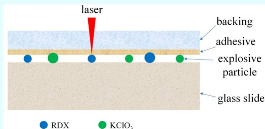
Figure 1: The diagram of identification of explosive particles on the adhesive side of the transparent tapes by laser confocal Raman microscopy.
