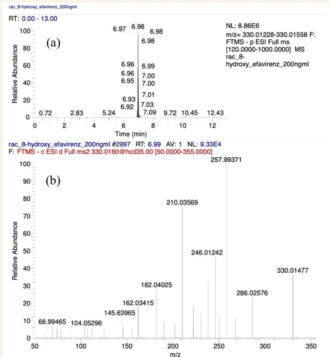
Figure 2. (a) Chromatogram and (b) ddMS2 spectrum of rac-8-hydroxy efavirenz at 200 ng/ml in LC-orbitrap-MS negative mode
