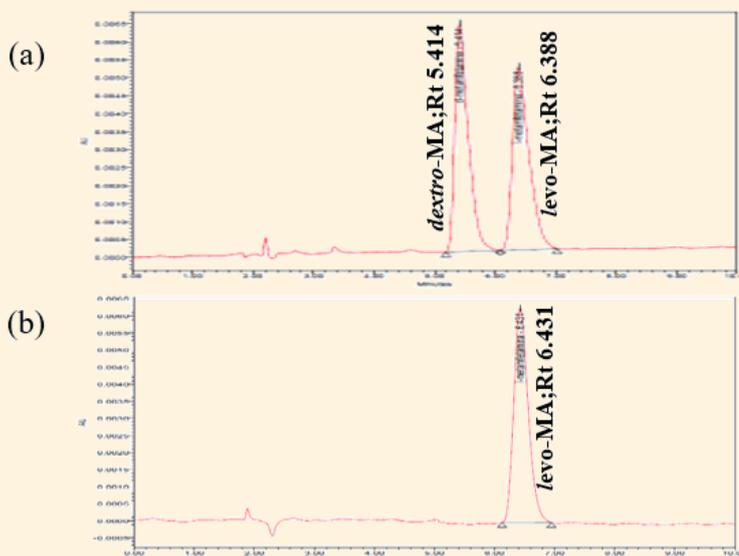
Fig. 3. Chirality analysis of (a) mixed of MA standards; (b) MA sample
