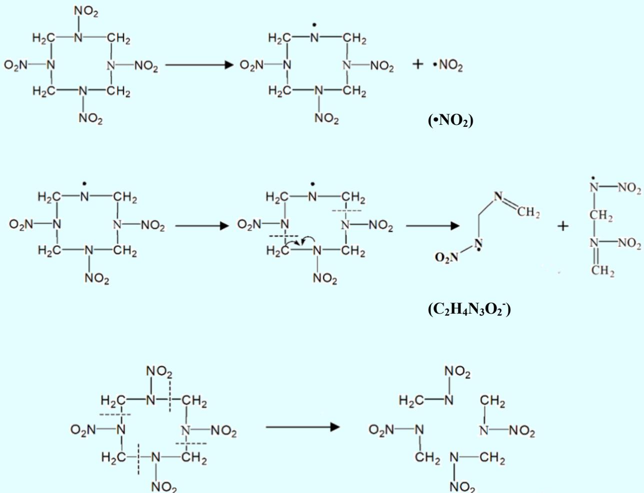
Figure 3. Proposed fragmentation pathway for the radical anions  $[M+NO_2]^-$  ( $m/z$  342) and  $[M+C_2H_4N_3O_2]^-$  ( $m/z$  398) of HMX.
