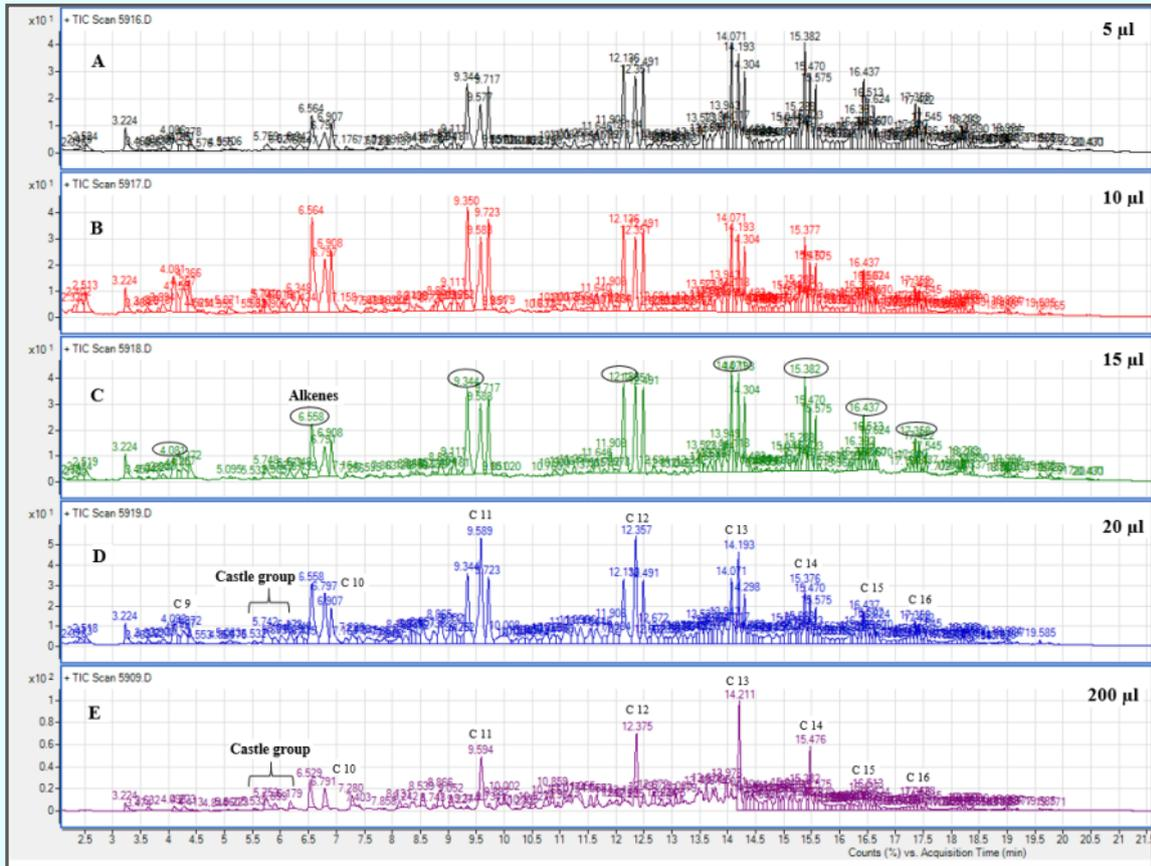
Figure 2: TICs for burnt PE samples spiked with kerosene of volume (A) 5 µl, (B) 10 µl, (C) 15 µl, (D) 20 µl and (E) 200 µl
