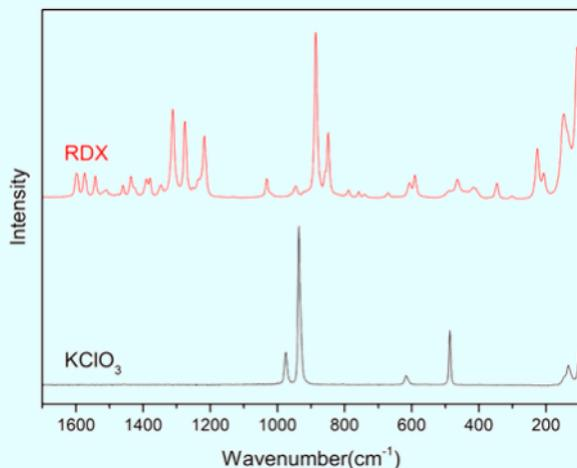
Figure 2: Raman spectra of RDX (above) and KClO<sub>3</sub> (below) particle
