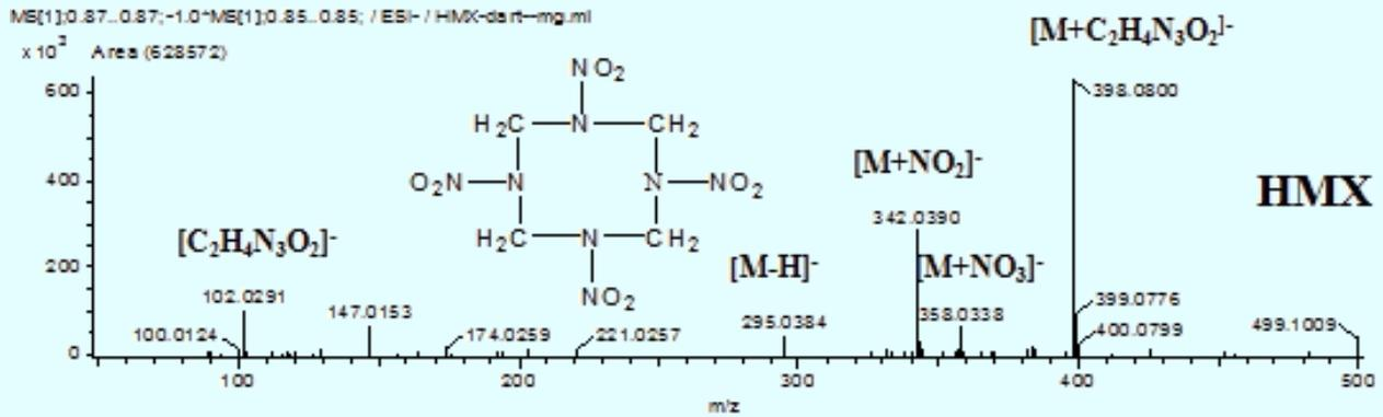
Figure 2. In-source CID TOF MS spectrum of HMX under DART negative mode by AccuTOF
