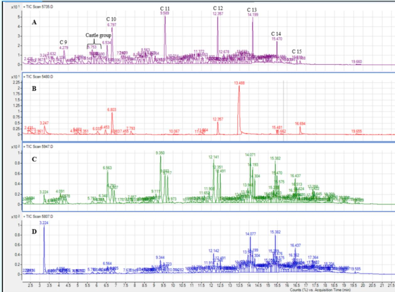
Figure 1: TICs for (A) 0.1% Kerosene reference, (B) Neat PE sample, (C) Burnt PE sample without kerosene and (D) Pyrolysed PE sample
